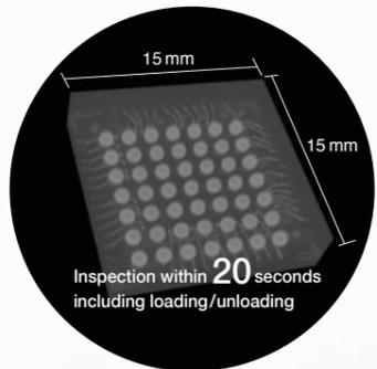
Visual inspection using fluoroscopic x-ray systems
