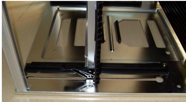
Quick release and guide rail
